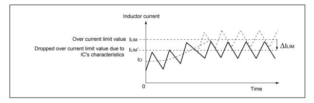
The over current detection value needs to set a sufficient margin against the maximum load current.
