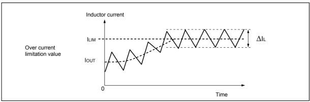
If the rate of inductor saturation current is small, the inductor value decreases and the ripple current of inductor increase when the over-current flows. At that time there is a possibility that the limited output current increases or is not limited, because the bottom of inductor current is detected. It is necessary to use the inductor that has enough large rate of inductor saturation current to prevent the overlap current.
