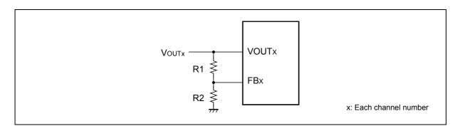
The total resistor value (R1+R2) of the setting output resistor should be selected up to  $100 \text{ k}\Omega$ .
